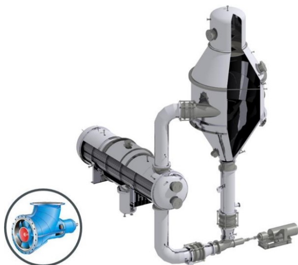
Figure 1 - An example of a Forced Circulation arrangement
